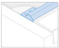
Diagram shows BCT16 butt jointed to the back edge of BG511 (5mm gauge - see page 39) stair edging to provide a neat edge to the carpet.
