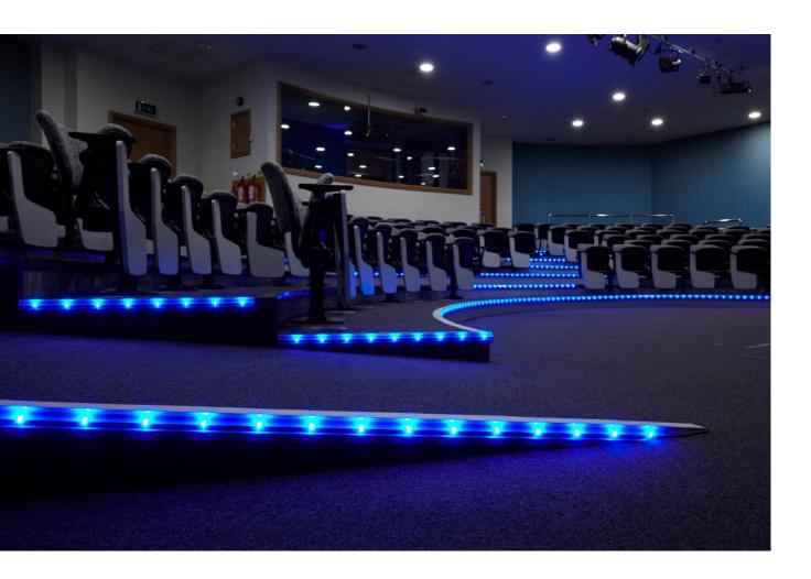
Gradus offers a range of safety and decorative lighting profiles for stairs. Profiles have been designed specifically to suit dark interior environments such as auditoria, where light is required for safety but should not detract from the primary function of the installation. By utilising LED technology, the system offers an extra low voltage (12v) alternative to mains voltage lighting.
