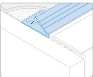
Diagram shows CG1042 butt jointed to the back edge of CT71 (gauge 7mm see page 31) stair edging to provide a neat edge to the carpet.
