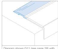
Diagram shows G11 (see page 28) with TA9 ramping strip providing a transition where no floorcovering is used.
