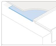
Diagram shows BU200 bevelled underlay being used to build up a 3.2mm linoleum to ensure a flush finish with the back edge of a G11 stair edging (5mm gauge - see page 28).
