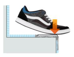
An insert provides a surface that creates friction between the sole of the shoe and the step edge, hence providing slip-resistance and reducing the risk of slips on stairs. All Gradus inserts are tested for slip-resistance – see results on page 159.
