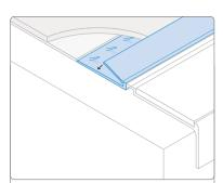
Diagram shows ANT355 butt jointed to the back edge of G11 (5mm gauge - see page 28) stair edging to provide a neat edge to the carpet.
