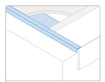
Diagram shows PET276 in conjunction with RN711 (gauge 6mm - see page 44) with a special on-site fabrication being used to protect the exposed edge of the carpet and form a 'carpet runner'.
