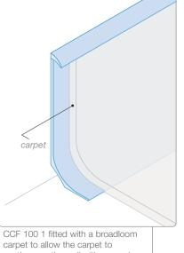
continue up the wall with a capping seal to protect the exposed edge.
